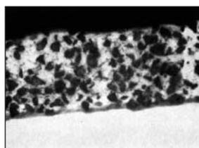
Fig. 1 — 1000X cross section photomicrograph of a EN/diamond coating with 2  $\mu$ m diamond particles.
