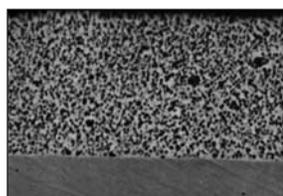
Fig. 2 — Cross section of EN/PTFE deposit.
