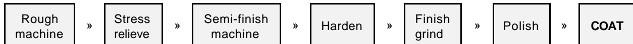
Figure 2 : Basic recommended pre-coating procedures. Each coating may also require additional steps as indicated in the text.
